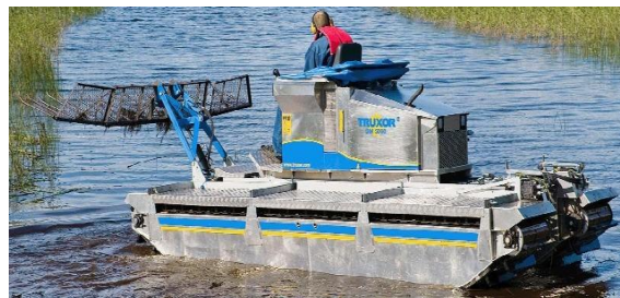
Fig.2 Multifunction boat for cleaning up the weeds
